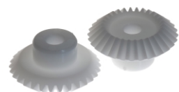
Part No. 919D25. Nylon Bevel Gears 1:1. OD30.7mm ID 6mm. Module 1.0. 6g
