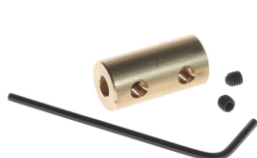
Part No. 919D1/8. In-line Coupling. 8mm-8mm Dia. 12.67mm x 24.8mm. 23g
